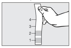
Dip the test strip in the water for 1 second and shake off any remaining water. The result is visible in about 1 minute.
